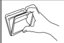
Remove the plastic insert by pivoting it on the bottom edge.
