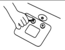
Tighten the mounting bolts.
