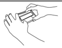
Squeeze the top edge of the black plastic insert down to release the top two locking tabs, carefully to prevent breakage.
