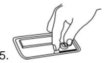
Now slide the POP&LOCK to the right so that the mounting bracket is positioned under the actuating rod on the passenger side.
