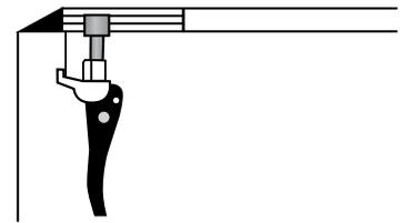
Rotate handle lever to locking position. Repeat for opposite side.
