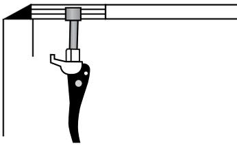
Rotate handle lever down from its storage position. Adjust clamps to proper height.
