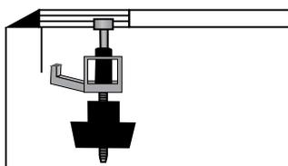
Adjust front slide-clamp to proper height.
