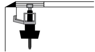
Rotate thumb nut to tighten clamp enough (not too tight).
