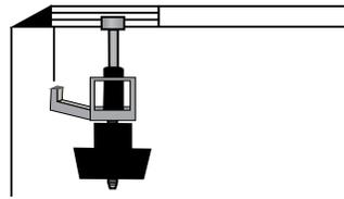
Slide front clamp holder under truck bed rail.
