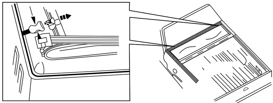
3. Unfold the cover completely and begin to adjust the rear EZ-Clamps at the rear of the bed. Again, make sure they are snug but **not tightened completely**. (Both front and rear clamps will be tightened completely in a later step.)
