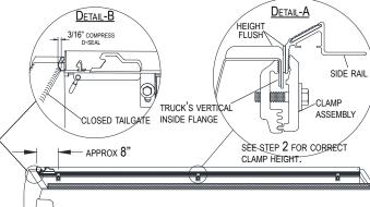
must be level. To adjust rails, loosen screws and reposition male clamps higher or lower. Tighten all clamps.
