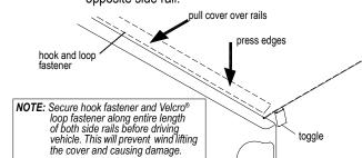
STEP 8: To release cover, Trigger pull rear release toggle. Start rolling cover toward cab making sure both sides of cover roll evenly. For best results leave unrolled portion of cover attached to the hook fastener and Velcro® loop fasteners while opening.
