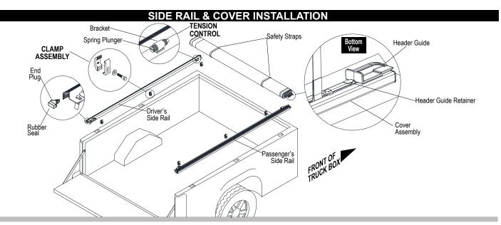
STEP 1: Attach the TruXedo rails to the truck's vertical inside flange as ISTEP 2: For optimum latching performance and cover fit, side rails shown in Detail A. To get the correct TruXedo rail alignment from front to back, See Detail-B. Compress the rear D-seal against the closed tailgate and hold. Attach clamps starting at the tailgate. Evenly space 3 clamps along each TruXedo rail, leaving approximately 8" on each end.
