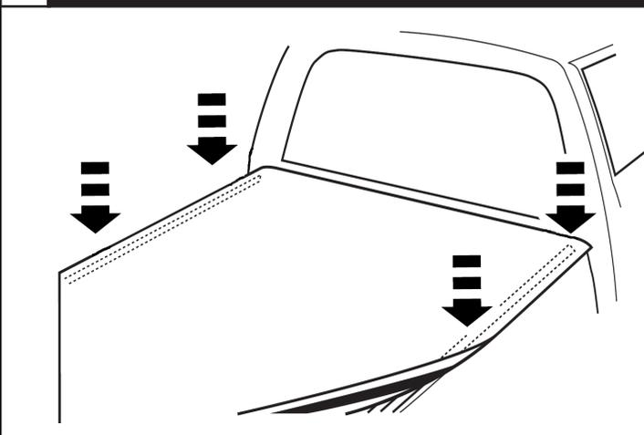
**Note:** Small wrinkles may be present after closing cover for first time. Remove wrinkles by pulling cover material from each side. For best results have cover unlatched. Relatch rear header after adjustments have been made.
