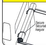
Before driving with cover open, BOTH STRAPS MUST BE SECURED TO RETAINING LOOPS. Failure to do so could cause accidental release of the cover, resulting in personal injury or property damage.
