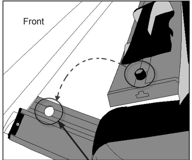
Note: The Pro X15 rail may need to be tilted upward slightly to allow the screw head to drop into the slot.
