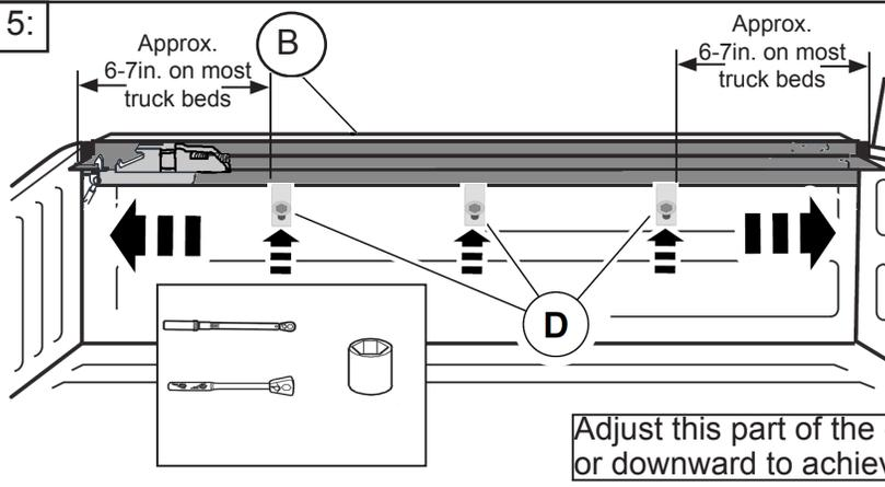
Adjust this part of the clamp upward or downward to achieve a level rail.
